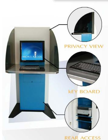
The K-Carrel is a "sit-down" designed model so that the user can relax while performing tasks such as application/form fill, browsing information, and signing documents. This unit can come with a laser printer that delivers the print to the user from just under the display.
